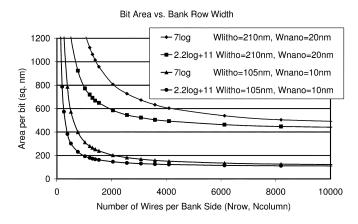
Fig. 5. Raw memory bit density as a function of  $N_{row}$ .
