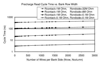
Fig. 8. Precharge read cycle time as a function of  $N_{row}$  for various resistances.  $W_{\text{litho}} = 105 \text{ nm}, W_{\text{nano}} = 10 \text{ nm}, 7 \lceil \log_2(N) \rceil$  addressing.
