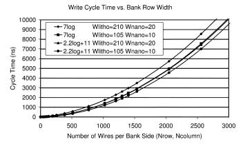
Fig. 6. Random write cycle time as a function of  $N_{\rm row}$  with  $R_{\rm contact}$  =  $1 \text{ M}\Omega$  and  $R_{\text{ondiode}} = 0.1 \text{ M}\Omega$ .
