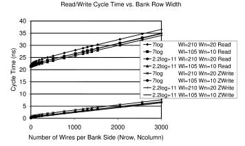
Fig. 7. Precharge read and zero write cycle time as a function of  $N_{\rm row}$  with  $R_{\text{contact}} = 1 \text{ M}\Omega \text{ and } R_{\text{ondiode}} = 0.1 \text{ M}\Omega.$
