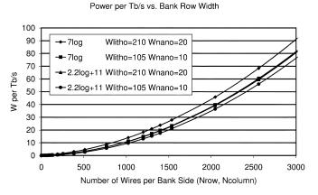
Fig. 10. Random write power per Tb/s a function of  $N_{row}$ .
