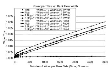
Fig. 9. Power per Tb/s a function of  $N_{row}$  for precharge read and zero write.
