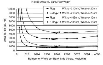
Fig. 12. Net memory bit density as a function of  $N_{\text{row}}$  ( $P_c = 0.95$ ,  $P_{\text{junc}} = 0.9999$ ,  $P_{\text{gbit}} = 0.95$ ,  $P_{\text{bank-yield}} = 0.98$ ).
